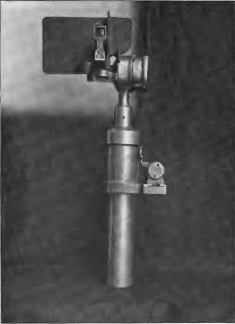
GONIOMETER (FRENCH) FOR TRAINING GUNS IN AZIMUTH.
